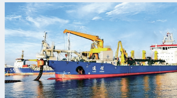
CCCC Tianjin Dredging 13,000 m 3 Trailing Suction Hopper Dredger
